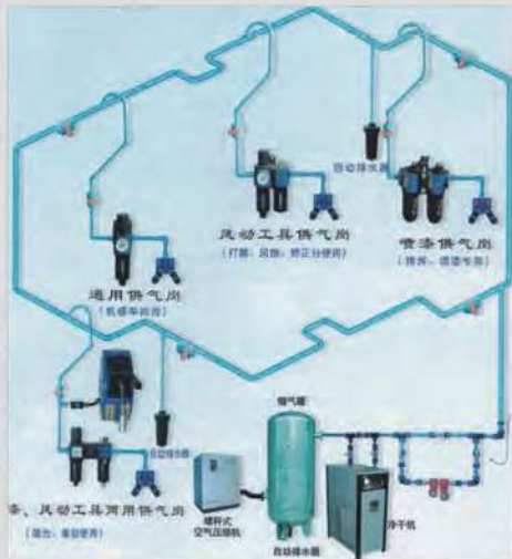
AIR SUPPLY SYSTEM DESIGN AND INSTALLATION
